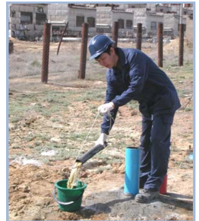
Groundwater well purging to obtain representative sample
