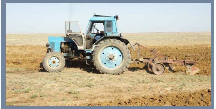
EcoSocio Analysts' Soil Bio-remediation by landfarming at a PreCaspian Region Oil Field. Soil aeration by ploughing.
