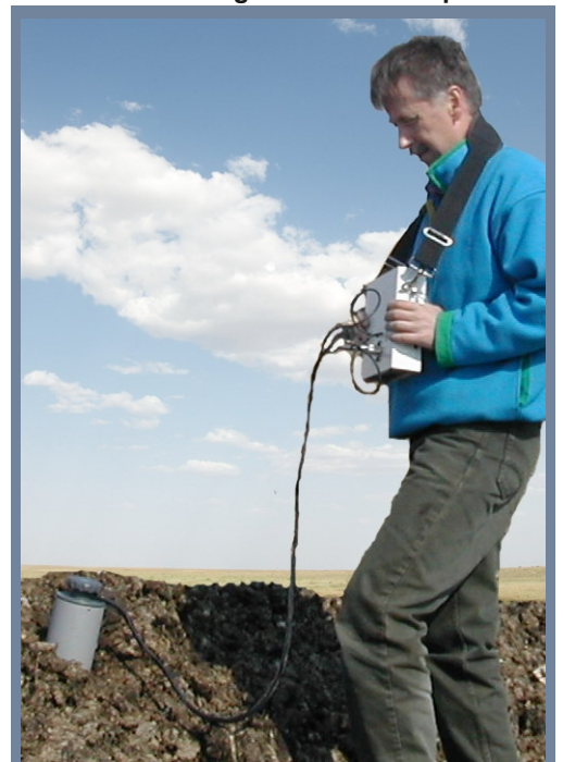
Measuring bacterial activity via soil CO 2 respiration rate and soil temperature change
