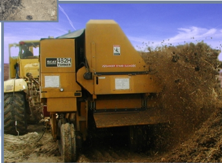
Aeration of the heavily contaminated soil and oil sludge arranged in windrows at Uzen Oil Field
