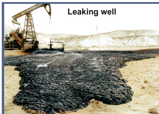
Sand massive on the Emba River Flood Plain is unprotected from oil over spills from a temporary storage tank during well development
