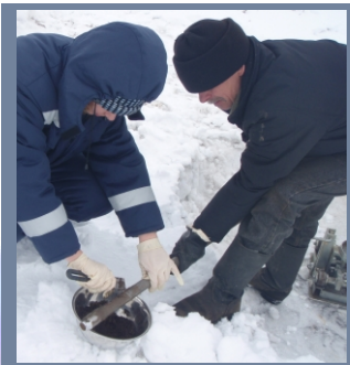
Ground and groundwater contamination analysis at an old municipal dump for construction of a large retail centre
