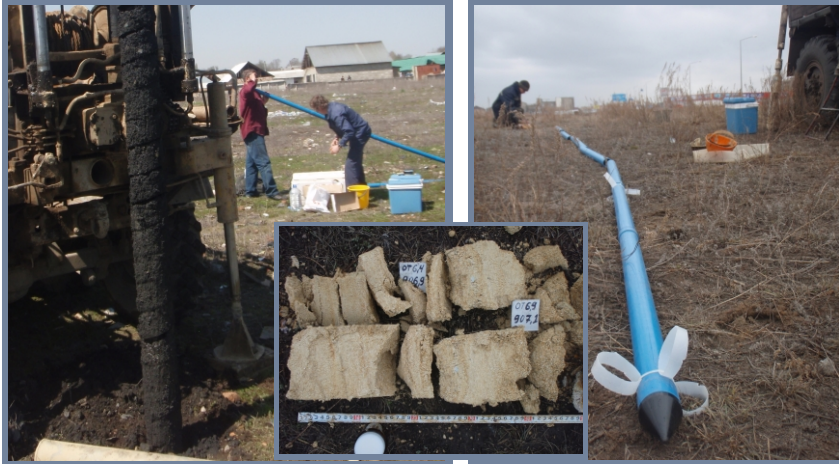
Ground and groundwater contamination analysis at an old municipal dump for construction of a large retail centre
