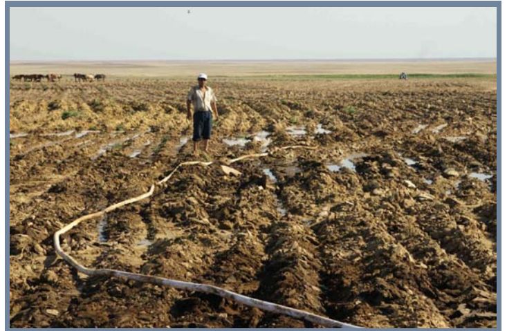
Maintaining the desired soil moisture is a challenge in the arid climate. Perforated hose watering the landfarmed plot
